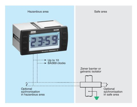
The BA369 is an intrinsically safe, battery powered, panel mounting digital clock that will accurately display local time in a hazardous area.
