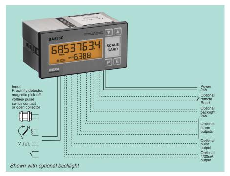
The BA538C is an externally powered rate totaliser with separate rate and total displays which will operate from a switch contact, voltage pulse, magnetic pick-off, open collector or a proximity detector input. A novel adaptive measuring technique plus an adjustable digital filter ensure that optimum rate display stability and step response can be achieved over a wide input frequency range.
